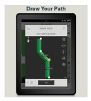
6. Press the Set button to save your profile and you're ready to start digging. Here's what a completed profile looks like on the Co-Pilot display.
